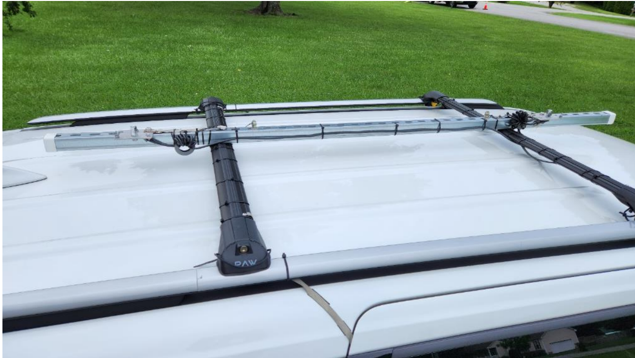
KIA Roof Rails, PAW Aluminum Roof Racks, and Galvanized Framing Strut (Lowes)
