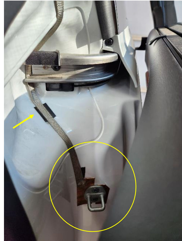
Braid Soldered to Copper Shims under each Sliding Door Striker Plate (4)
