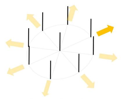
Outer element-to-center element spacing = 60 ft (Circle diameter = 120 ft)
