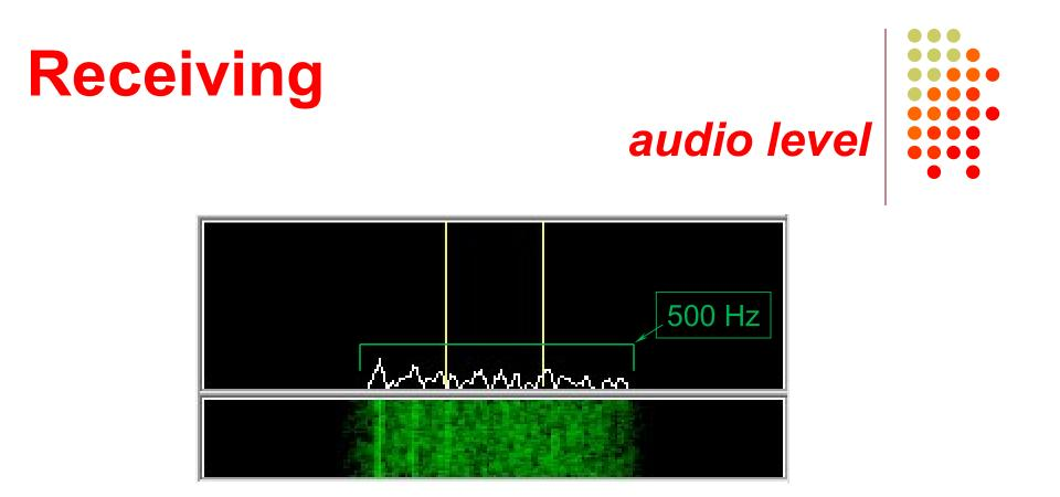
• Set RX audio level with no-signal at 5% of full-scale
