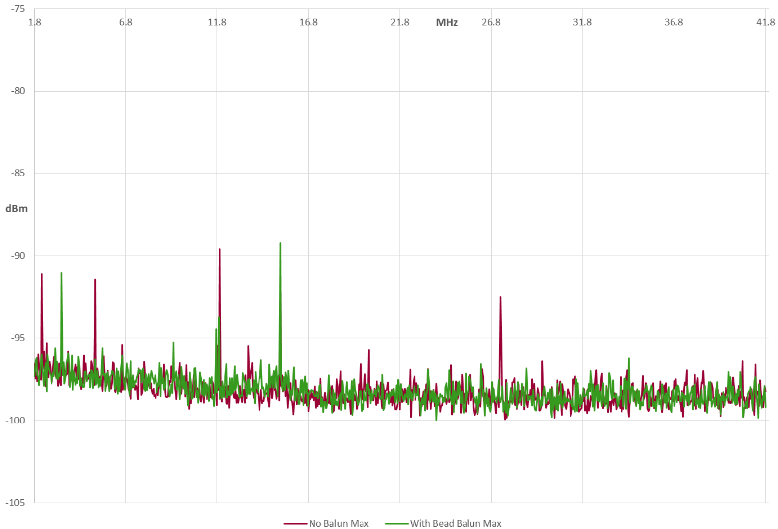
Tower 2 Current Probe Measurements w/ 18 dB Attenuation
