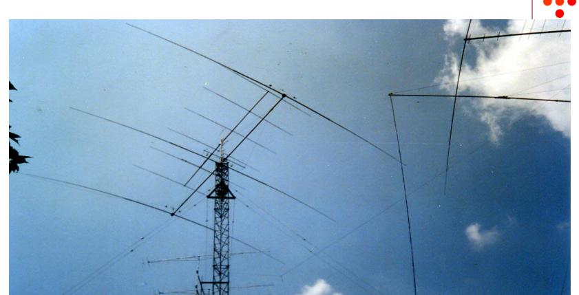
K3ZO's very successful horizontally polarized 3 element Yagi changed my thinking about 80 meter antennas for DX
