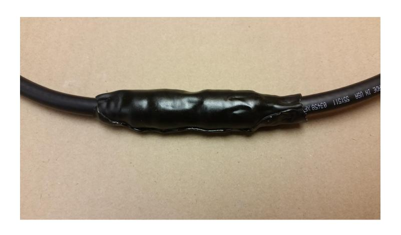
Two wraps of 88 tape. Overlap each layer by ½ the width of the tape.
