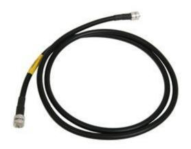
When soldering PL259's, don't be afraid to use a big iron and get the connector hot — the solder must flow. Just keep everything straight in-line and be sure to let it cool down completely before you move it. That way the center dielectric will harden back up. I let mine sit about 10 minutes after soldering before doing anything with it.
