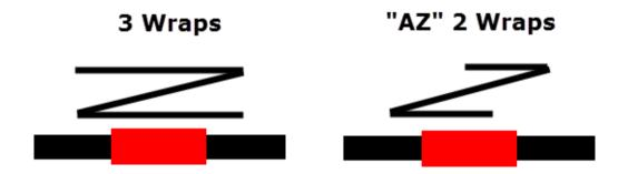
The "AZ" design is two wraps that leaves the tape end in the middle of the junction to make finding it easier in the future (source: Ohio Bell).
