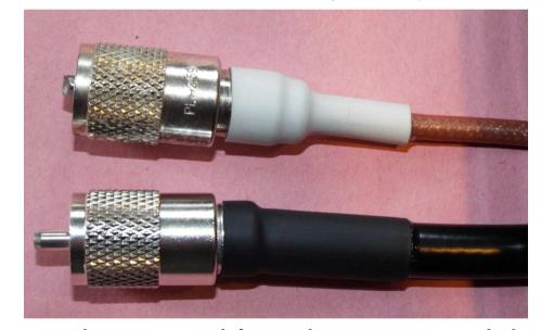
Be sure that you trust the assembler, since you can't back off the shell to check the body solder holes.
